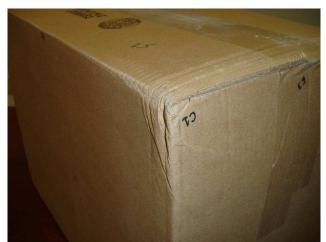
Figure 20 - sm130 handling drop test, packaged equipment, typical damage, corner C1
