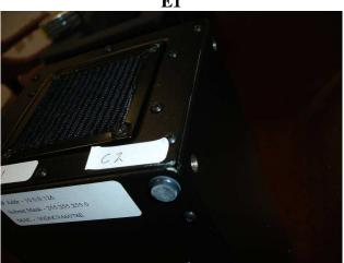
Figure 25 – sm130 handling drop test, unpackaged equipment, typical damage, corner C2
