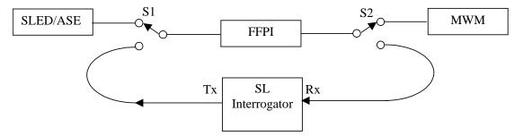
Figure 7: Block Diagram of Test Configuration
