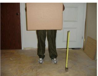
Figure 13 – sm130 handling drop test, packaged equipment, surface S1
