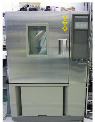
Figure 9. Espec environmental chamber used for testing.
