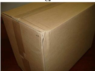
Figure 22 - sm130 handling drop test, packaged equipment, typical damage, corner C3
