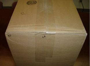
Figure 19 - sm130 handling drop test, packaged equipment, typical damage, edge E3
