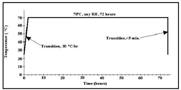
Figure 2. High Temperature Thermal Shock
