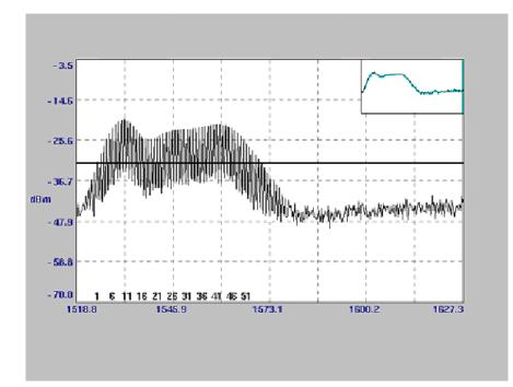
Figure 11. Calibration and test optical artifact as seen by reference instrument
