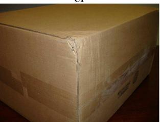
Figure 21 - sm130 handling drop test, packaged equipment, typical damage, corner C2
