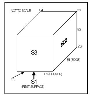
Figure 5. Drop Surfaces for Handling Test - Packaged Container
