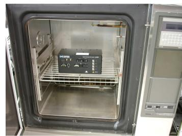
Figure 10. EUT inside test chamber.
