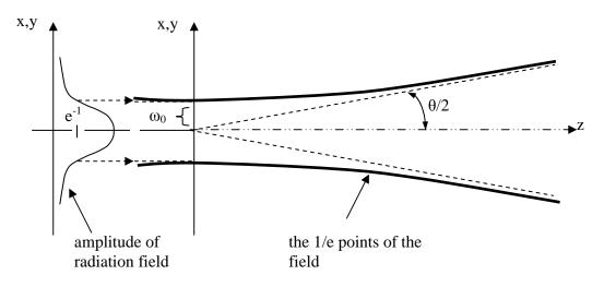
Figure 27. Beam divergence of  $TEM_{0,0}$  mode from single mode fiber.
