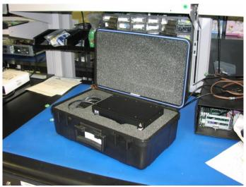
Figure 15. sm125 and carrying case unaffected by drop tests.
