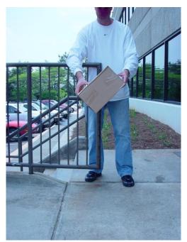
Figure 13. Packaged Drop Test – edge 3
