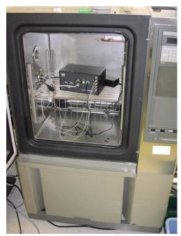
Figure 10. EUT inside test chamber.
