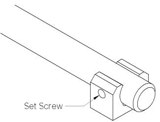
Figure 3 – Close up of mounting bracket & Setting Bar
