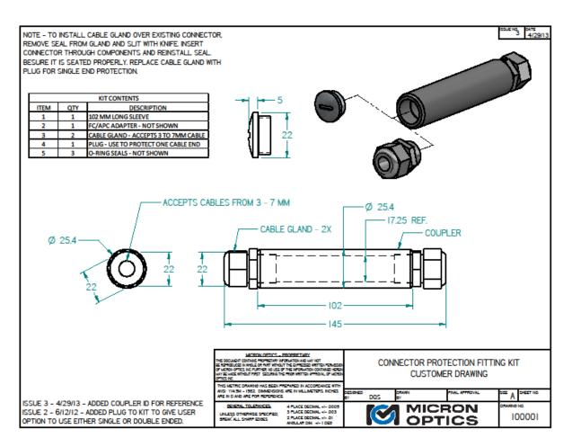
Figure 18 – Universal Connector Protection Fitting
