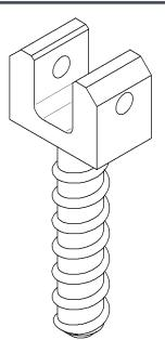
Figure 6 – Concrete Mounting Bracket
