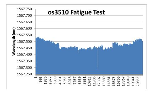
**Conclusion**: No failures were found during fatigue testing. The test was concluded when the test fixture was needed for another product test.
