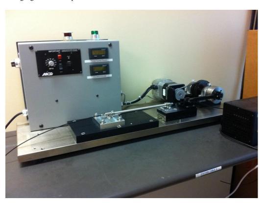
While exercising the strain sensor, the wavelength (WL) of the strain and temperature FBG were captured using a Micron Optics sm130. The strain FBG WL data is basically a sign wave as the sensor is extended from minimum strain to maximum strain.
