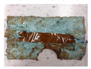
Figure 6 – Removed STOPAQ
