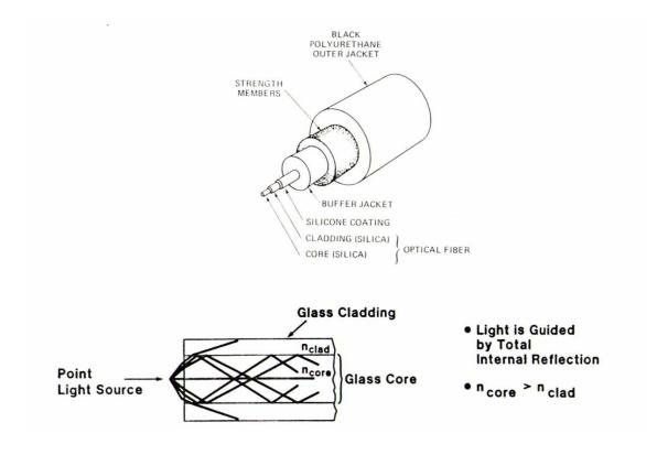
**Figure 2.1**: Schematic of an optical fiber.
