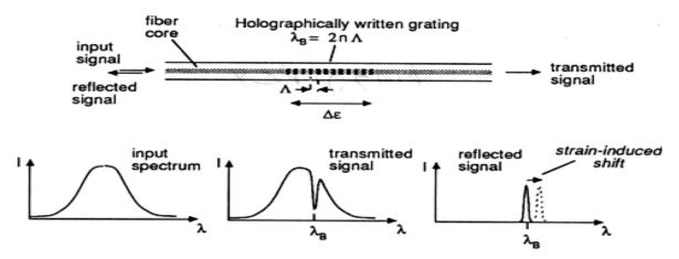
Figure 3.1. Transmission and reflection spectra of a fiber Bragg grating
