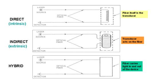
Figure 2.3: Classification of optical fiber sensors
