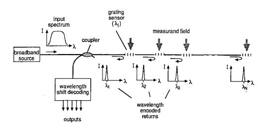
Figure 3.4 Schematic representation of a WDM interrogation of a FBG array
