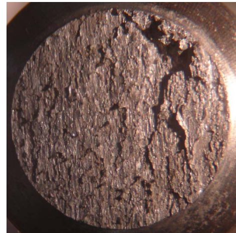
Figure 14. UNS A95083 fracture sample shows a predominate region of SCC along with a small region of ductile overload in the upper right of the crack tip.
