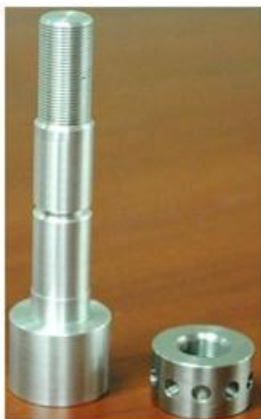
Figure 4. Circumferentially V-notched fracture mechanics sample and load nut.
