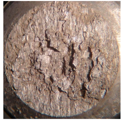
Figure 18. UNS A95083 fracture sample crack tip shows SCC cracking with areas of ductile overload in the center.
