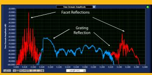
The time domain response clearly shows the large facet reflections and grating reflection of the silicon photonic waveguide.
