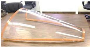
Luna's hydrophobic coating on an F-16 canopy.
