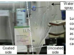
Luna's hydrophobic coating exhibits superior watershed as compared to currently used canopy coatings.
