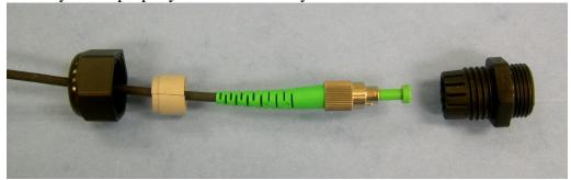
7. (Note that while you are slitting the seal you can use a 13.5 mm pin to spread the teeth of the body apart. This will make it easier to insert the seal back into the body once on the cable.)
