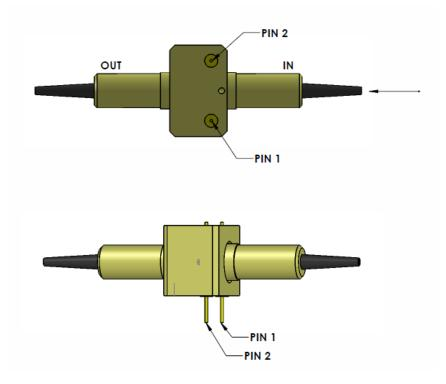
Figure 6 PSW-002 pinout
