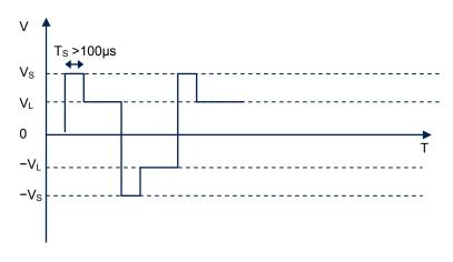
Figure 5 Drive signal diagram  $V_s$  = switching voltage  $V_L$  = latching voltage  $T_s$  = time switching voltage is applied
