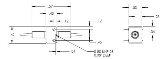
Figure 8 Dimensions and mounting hole information All dimensions given in inches.
