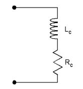
Figure 4 PSW-002 equivalent electrical circuit
