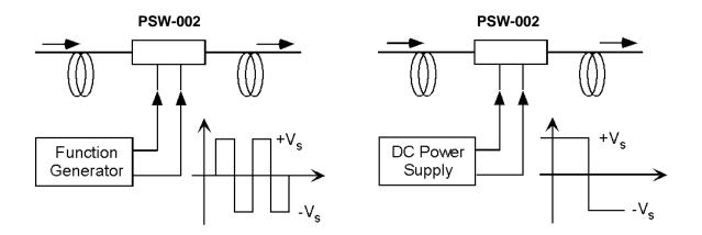
Figure 9 Examples of basic driver setups. A function generator can be used to drive the PSW for periodic switching, while a DC power supply may be sufficient for occasional switching. Note that this diagram shows only switching voltages. Once the device has switched state, the voltage can be lowered to the latching voltage to maintain the output state.
