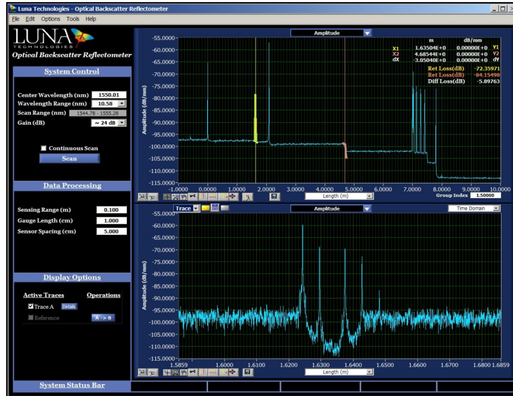
Figure 3-1. OBR control software main window, with data loaded. Note that the upper vertical cursors are on, so loss calculations are shown in the upper graph. The sensing features and shift reference displayed in the Data Processing and Display Options areas are not available on all OBR units. The number of traces available also depends on OBR configuration.
