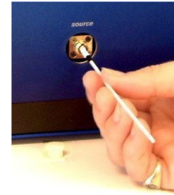
Figure 9-1. Remove the protective cap. Gently insert supplied mini swab, rotate in one direction, then remove.
