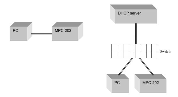
Figure 28 Direct connection: MPC-202 to PC
