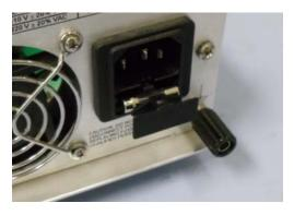
Figure 7 Fuse compartment
