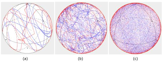
Figure 12 10-second capture of Rayleigh scrambling at (a) 10, (b) 100, and (c) 1000 rad/s mean SOP variation rate.
