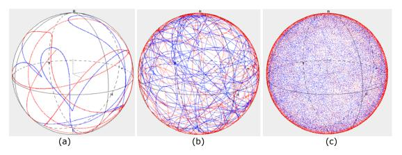
Figure 10 10-second SOP capture of triangle scrambling at rate = (a)  $1\times2\pi/s$  (b)  $10\times2\pi/s$ , and (c)  $100\times2\pi/s$ .
