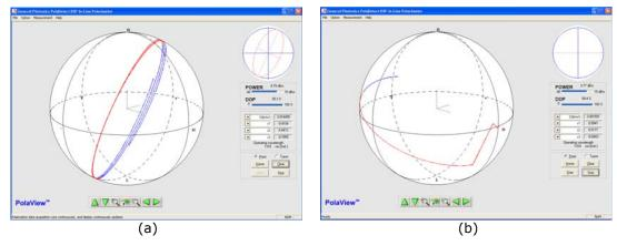
Figure 21 (a) 150V applied to channel 4. (b) Conversion of a random state to horizontal linear polarization
