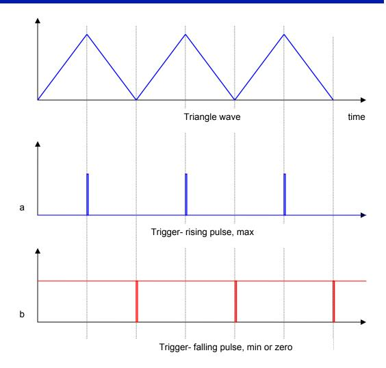
Figure 26 Output trigger examples
