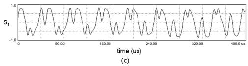
Figure 14 10 second SOP capture of tornado scrambling: (a) randomly rotating spin axis at 20 revolutions per second, (b) fixed rotating spin axis at 100 rev/s. (c) Tornado scrambling rate of 40,000 revolutions/s confirmed by measurement of one of the three Stokes parameters vs time, measured using the oscilloscope mode of a General Photonics polarimeter. The measured periodicity is 25µs per revolution, or 40,000 rev/s.
