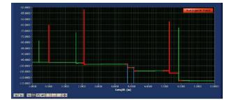
The Lightpath software compares the actual measurement parameters and compares the results to the user-defined parameter set. A determination of pass/fail is made and the results displayed on the user interface.
