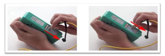
Figure 7-4 - Cleaning the Connector on the Tape
