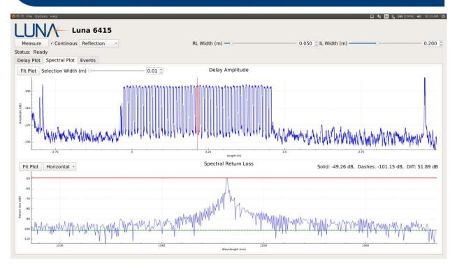
Figure 6-2 Spectral amplitude response plot showing the spectral amplitude of a single FBG
