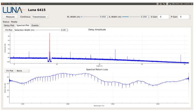
Figure 6-4 Transmission measurement of an optical network containing a gas absorption cell.
