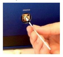
Figure 7-5 - Cleaning Optical Bulkhead Connections
