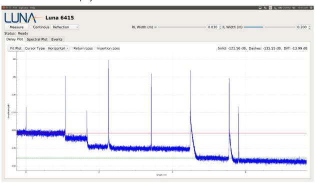
Figure 6-1 Reflection measurement of a fiber array
