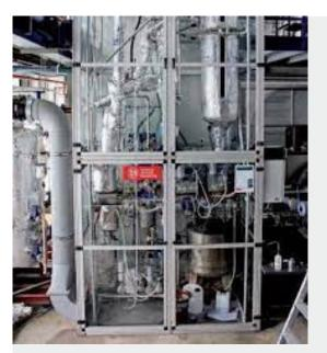
Heat Exchanger for Condensing Hexaol
