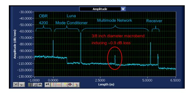
Figure 5. OBR 4200 scan of a multimode network branch using the Luna Mode Conditioner. Note the reflective signature at the fault makes locating it obvious since no reflections are expected between the input to the network and the receiver.
