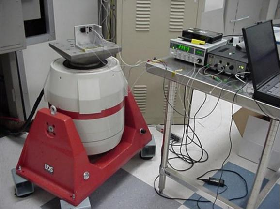
Figure 8: Vibration Table Setup
