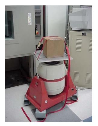
Figure 1: DUT in Shipping Box Strapped to Vibration Table
